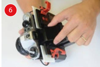
Adjusts the height of the focusing screen to the shutter.
