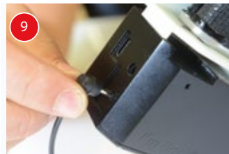
Connect the camera and the I'm Back® with the Sync Flash cable.
